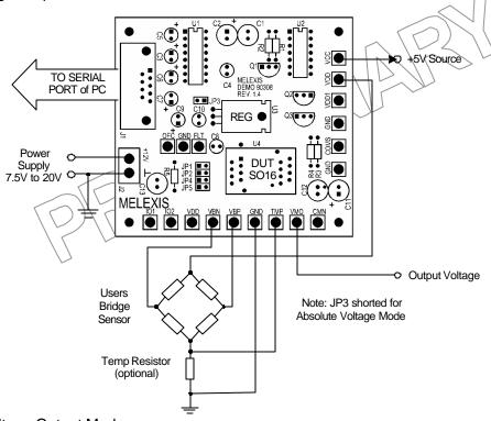
Ratiometric Voltage Output Mode:
